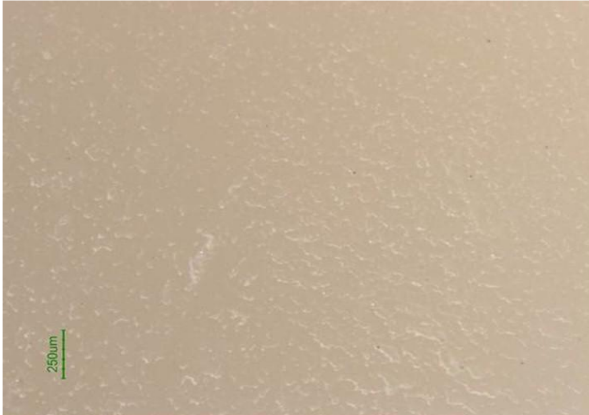
Figure 4. Scanning electron micrograph of the surface of group 3 where surface sealant (G-Coat Plus) was applied ( \times 1000 magnification).
